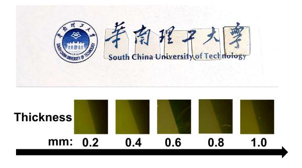
Fig. S16 Photographs of different thicknesses of glasses under daylight and modulated X-ray imaging, respectively.
