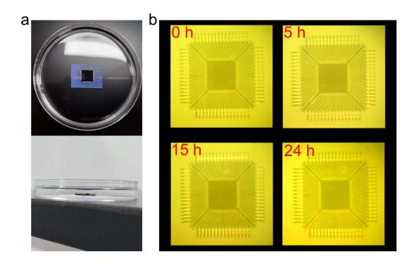
**Fig. S18** (a) Top view (top) and side view (bottom) photographs of the AI chip and Cs<sub>3</sub>MnBr<sub>5</sub> NC-embedded glass soaked in deionized water. (b) X-ray images of the AI chip in deionized water with storing times up to 24 h.
