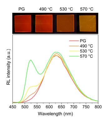
Fig. S12 Photographs (top) and RL spectra (bottom) of the PG and the glass sample annealed at different annealing temperatures for 5 h under X-ray excitation with a dose rate of  $4.814 \text{ mGy}_{air} \text{ s}^{-1}$ .
