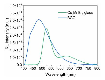
Fig. S11 RL spectra of BGO and  $Cs_3MnBr_5$  NC-embedded glass. The light yield of BGO is ~ 10000 photons MeV<sup>-1</sup>, therefore, the light yield of  $Cs_3MnBr_5$  NC-embedded glass is estimated to ~ 5200 photons MeV<sup>-1</sup> by comparing their RL integral area.<sup>42</sup>
