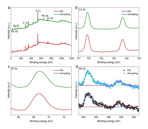
Fig. S2 (a-d) X-ray photoelectron spectroscopy (XPS) survey scan (a), and high-resolution XPS spectra of Cs (b),
