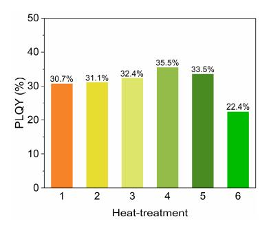
Fig. S7 PLQY recorded under 365 nm light excitation for the glass sample heat-treated at 490  $^{\circ}$ C (1) and 530  $^{\circ}$ C
