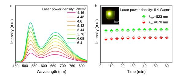
**Fig. S10** (a) PL spectra of the glass sample annealed at 570 °C for 5 h at different laser power densities. (b) Timedependent emission intensity of the corresponding sample under continuous excitation at 6.4 W/cm<sup>2</sup> power density for 1 h. The excitation wavelength used in (a, b) is 375 nm.
