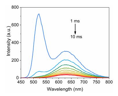
Fig. S5 Time-resolved PL spectra recorded from 1 ms to 10 ms following pulse excitation for the glass sample
