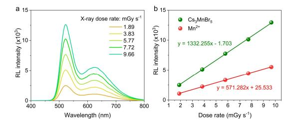
Fig. S13 (a, b) RL spectra (a) and liner relationship between dose rate and RL intensity (b) of  $Cs_3MnBr_5$  NCs and  $Mn^{2+}$  in glass at different dose rates under X-ray excitation.
