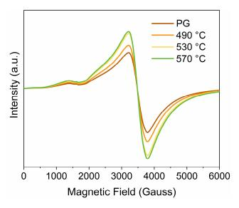
Fig. S3 EPR spectra recorded at room temperature for the glass sample annealed at different annealing temperatures.
