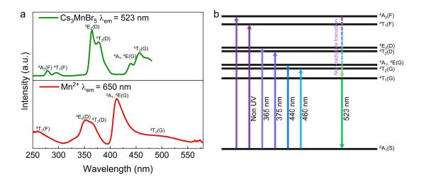
Fig. S4 (a) PLE spectra of Cs<sub>3</sub>MnBr<sub>5</sub>NCs and Mn<sup>2+</sup> ions in glass annealed at 570 °C for 5 h. (b) Schematic diagram
