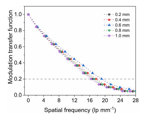
Fig. S17 MTF of X-ray images obtained from the different thicknesses of glasses.
