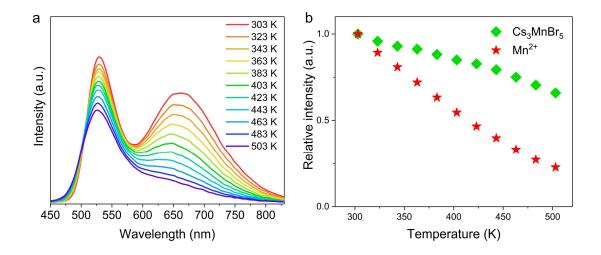
**Fig. S9** (a, b) Temperature-dependent PL spectra (a) and emission intensity as a function of measurement temperature (b) for the glass sample annealed at 570 °C for 5 h under 375 nm laser excitation.
