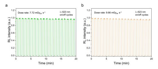
Fig S20 RL intensity of Cs<sub>3</sub>MnBr<sub>5</sub> NCs in the glass recorded under different dose rates over continuous 20 on/off cycles during 20 min.
