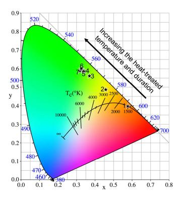
**Fig. S8** Chromaticity coordinates for the PL from the glass samples heat-treated at various temperatures and durations. The excitation wavelength used in the Commission Internationale deL'Eclairage (CIE) 1931 diagram is 365 nm. The glass samples were heat-treated at 490 °C (1) and 530 °C (2) for 5 h, and 570 °C for 5 h (3), 10 h (4), 20 h (5) and 40 h (6).
