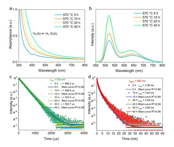
Fig. S6 (a-d) Absorption spectra (a), PL spectra (b) and PL decay curves of  $Cs_3MnBr_5 NCs$  (c) and  $Mn^{2+}$  ions (d) for the glass sample annealed at 570 °C for different durations. The fitting curves are fitted with single-exponential
