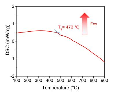
**Fig. S1** Differential scanning calorimetry (DSC) curve of the PG. According to DSC, it can be found that the glass transition  $(T_g)$  temperature of the glass sample is 472 °C. Due to the small size and volume fraction of the Cs<sub>3</sub>MnBr<sub>5</sub> NCs formed in the glass matrix, no obvious crystallization peak was observed. Therefore, we conducted a series of annealing precedures on the glass at temperatures higher than 490 °C.
