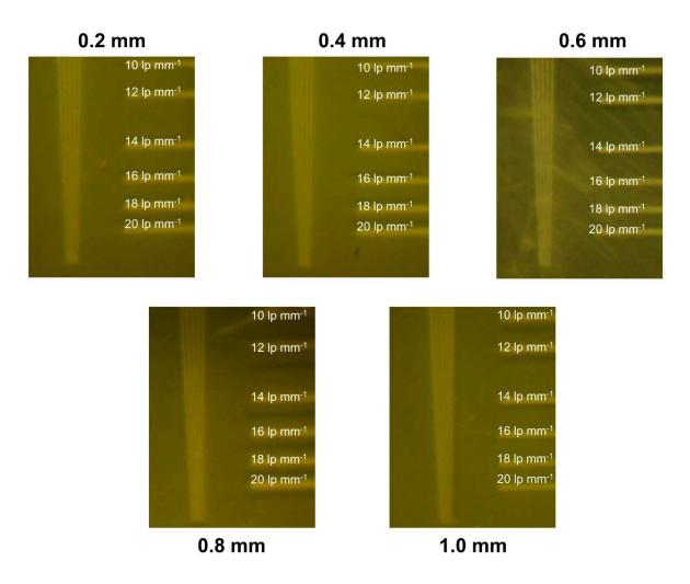
Fig. S15 X-ray images of the standard X-ray resolution pattern plate with different thicknesses of glasses.
